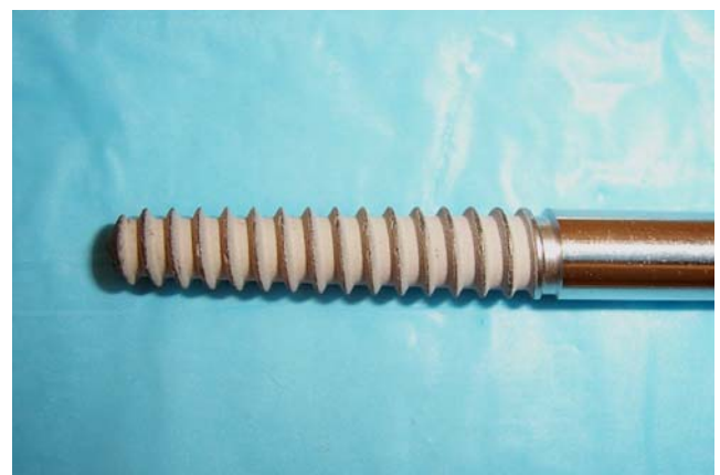
Fig. 21. Typical hydroxyapatite (HA) coated, 5–to–6 mm tapered half pin. This would be used in the adult tibia, femur and humerus
