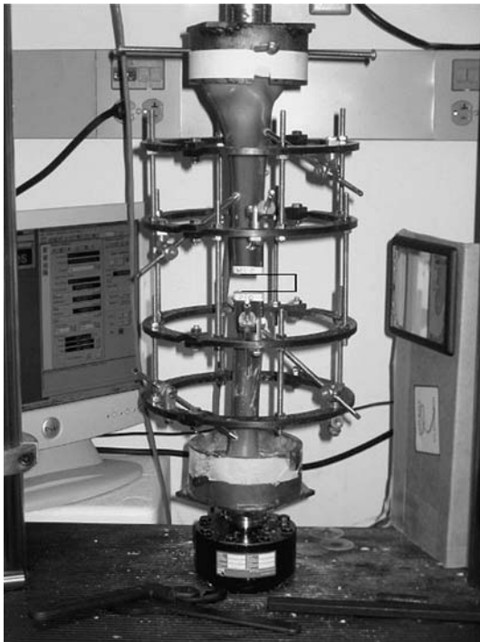
Fig. 5 A divergent frame with simulated 2-cm fracture gap (black rectangle seen at midshaft) was mounted in an MTS machine with biplanar video imaging to determine the strain of each construct.
